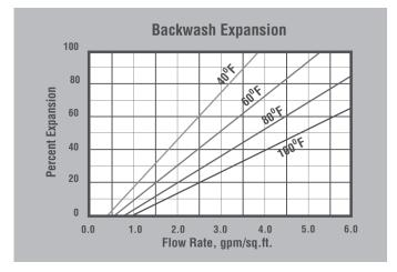
**BACKWASH** — The backwash step is used to separate the components prior to regeneration and to remove particles. The separation is optimized at a bed expansion of 50 to 75 percent.
